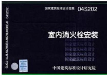
paperback. Book Condition: New. Paperback Pages Number: 36 Language: Chinese. 04S202 indoor fire hydrant installation suitable for industrial and civil indoor fire hydrant installation. Applies to brick walls. concrete walls. installation of fire hydrant on a variety of lightweight partition and bolt box fixed. Installation. including equipment. concealed. semi-concealed.
